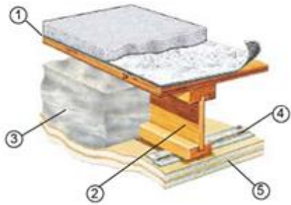
FIGURE 1 — SOUND RATED ASSEMBLY INCORPORATING WOOD I-JOISTS
