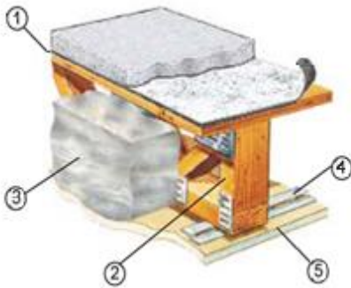
FIGURE 2 — SOUND RATED ASSEMBLY INCORPORATING WOOD TRUSSES
