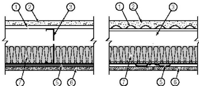
**1. Steel Deck** — Min 9/16 in. deep, 22 MSG galv corrugated fluted steel deck. Overlapped one corrugation at each side and attached to each joist with 3/4 in. long #10-16 TEK screws 10 in OC max.
