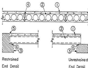
**1. Finish Flooring-Floor Topping Mixture\*** — 3 to 7 gal of water mixed with 80 lbs of floor topping mixture and 1.0 to 2.1 cu ft of sand. Compressive strength to be 1000 psi min. Min thickness to be 3/4 in. **MAXXON CORP** — Type D-C, GC, GC 2000, L-R, T-F, CT. Or — 4 to 7 gal of water mixed with 80 lbs of floor topping mixture and 1.4 to 1.9 cu ft of sand. Compressive strength to be 1200 psi min. Min thickness to be 3/4 in. **RAPID FLOOR SYSTEMS** — TYPE RF, RFP, RFU, RFR, Ortercrete
